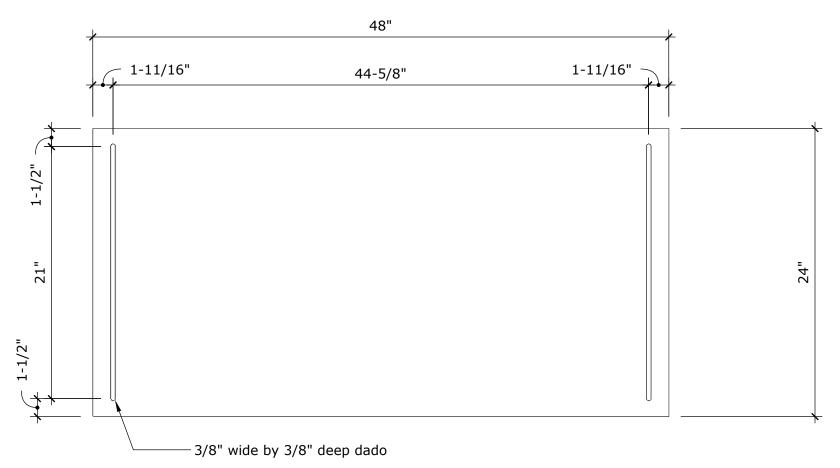
note: overall dimension can be smaller to accommodate smaller sheet sizes, maintain dado length and spacing
